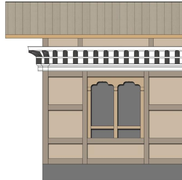
Fig.2.4.d.SINGLE STOREY SHAMIG WITH ONE LAYER OF BOGH AND PHANA
