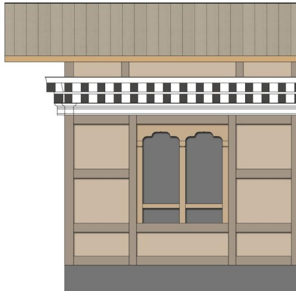
Fig.2.4.c.SINGLE STOREY SHAMIG WITH TWO LAYERS OF BOGH
